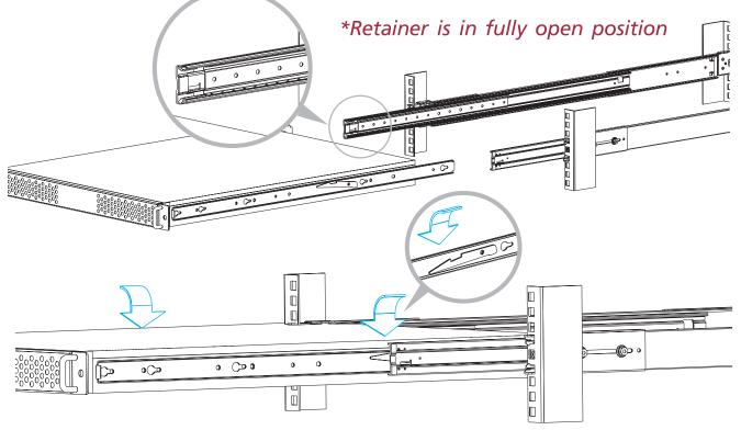
\*Press trigger down to release the slides from locking
