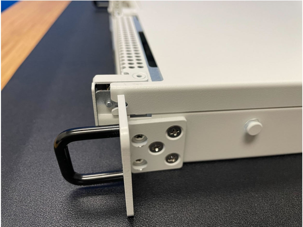
Fig. 6: Sliding back the top cover away from the front panel
