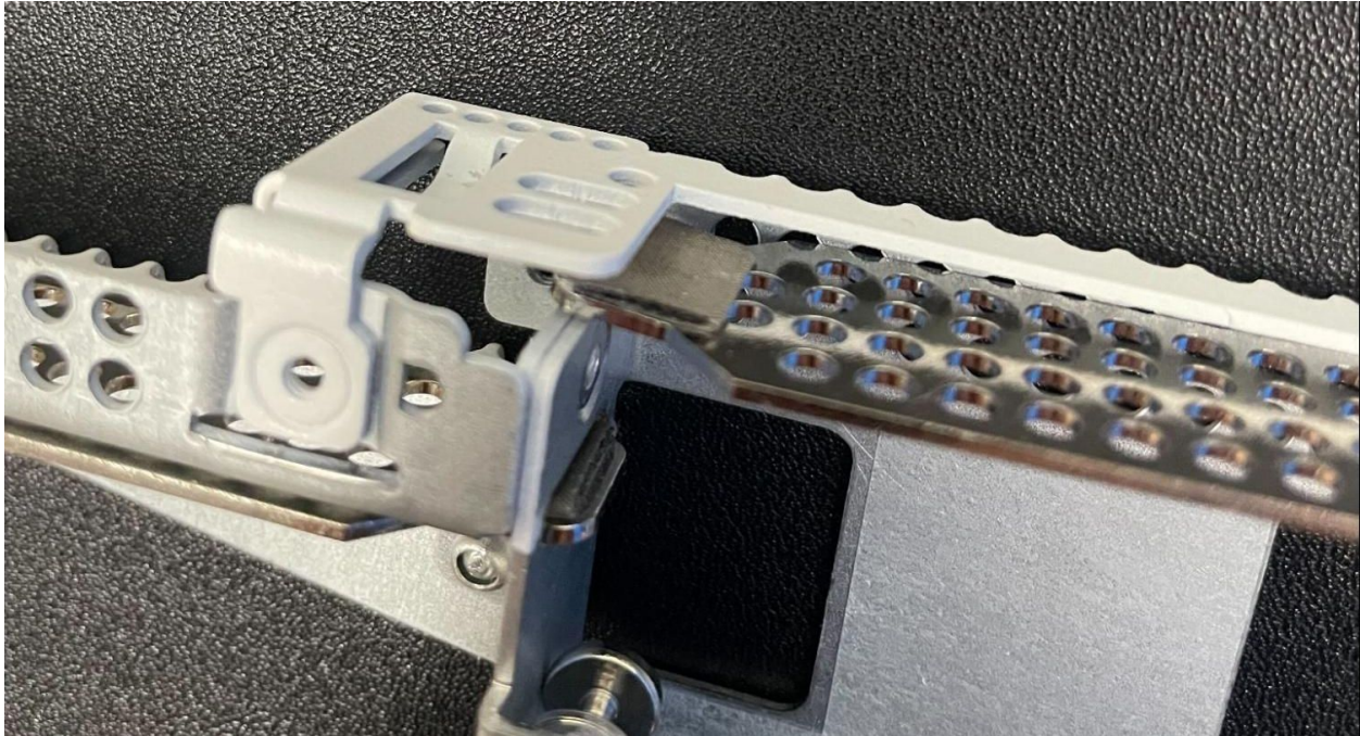
Fig. 16: Remove the expansion slot cover once it is free from the expansion slot
