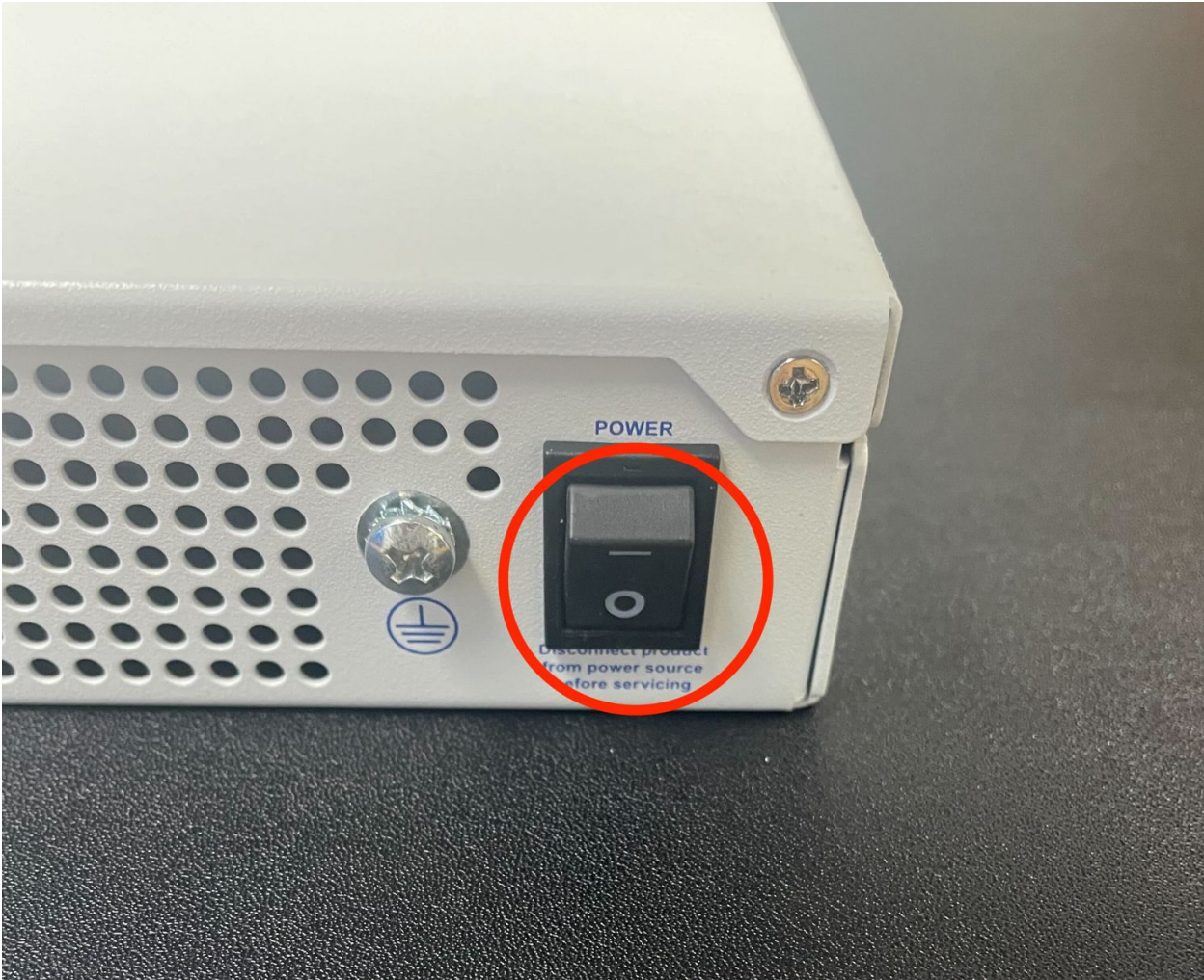
Fig. 1: Power switch (circled) in the off position
