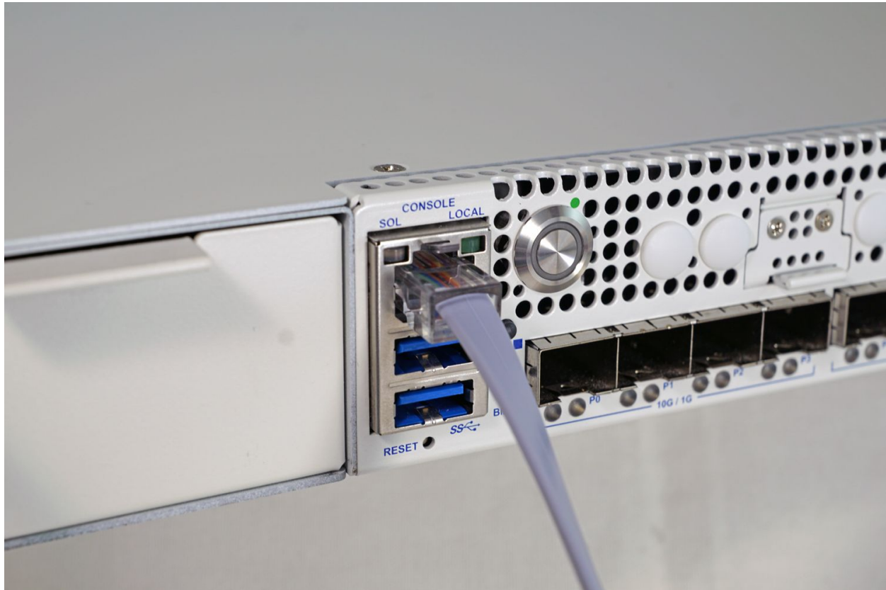
Fig. 1: Serial cable connected to RJ45 Console Port
