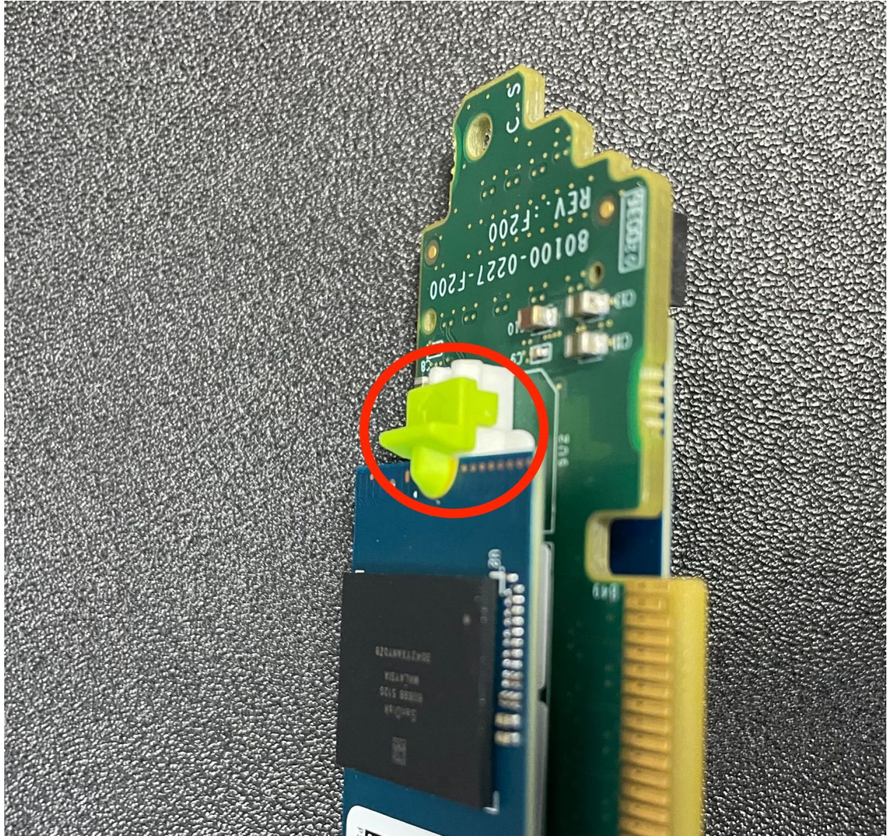
Fig. 15: Close-up view of the M.2 retaining clip for slot 2 with the SSD secured
