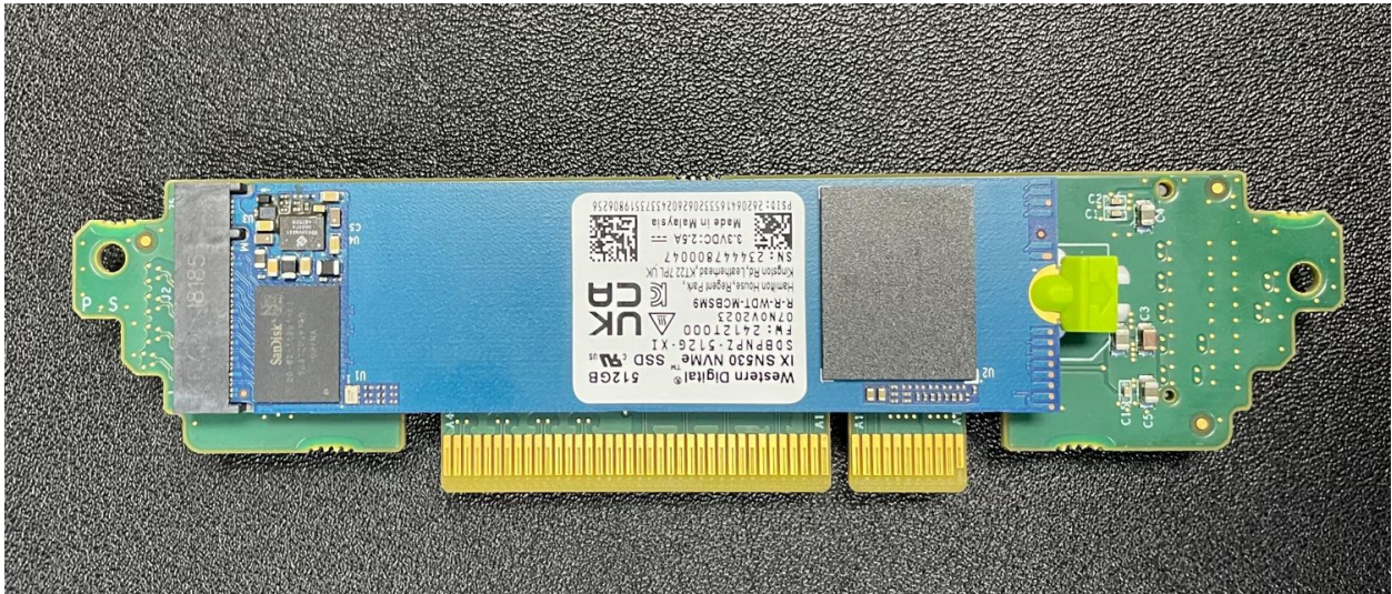
Fig. 12: M.2 NVMe riser card slot 1 with the stock SSD installed
