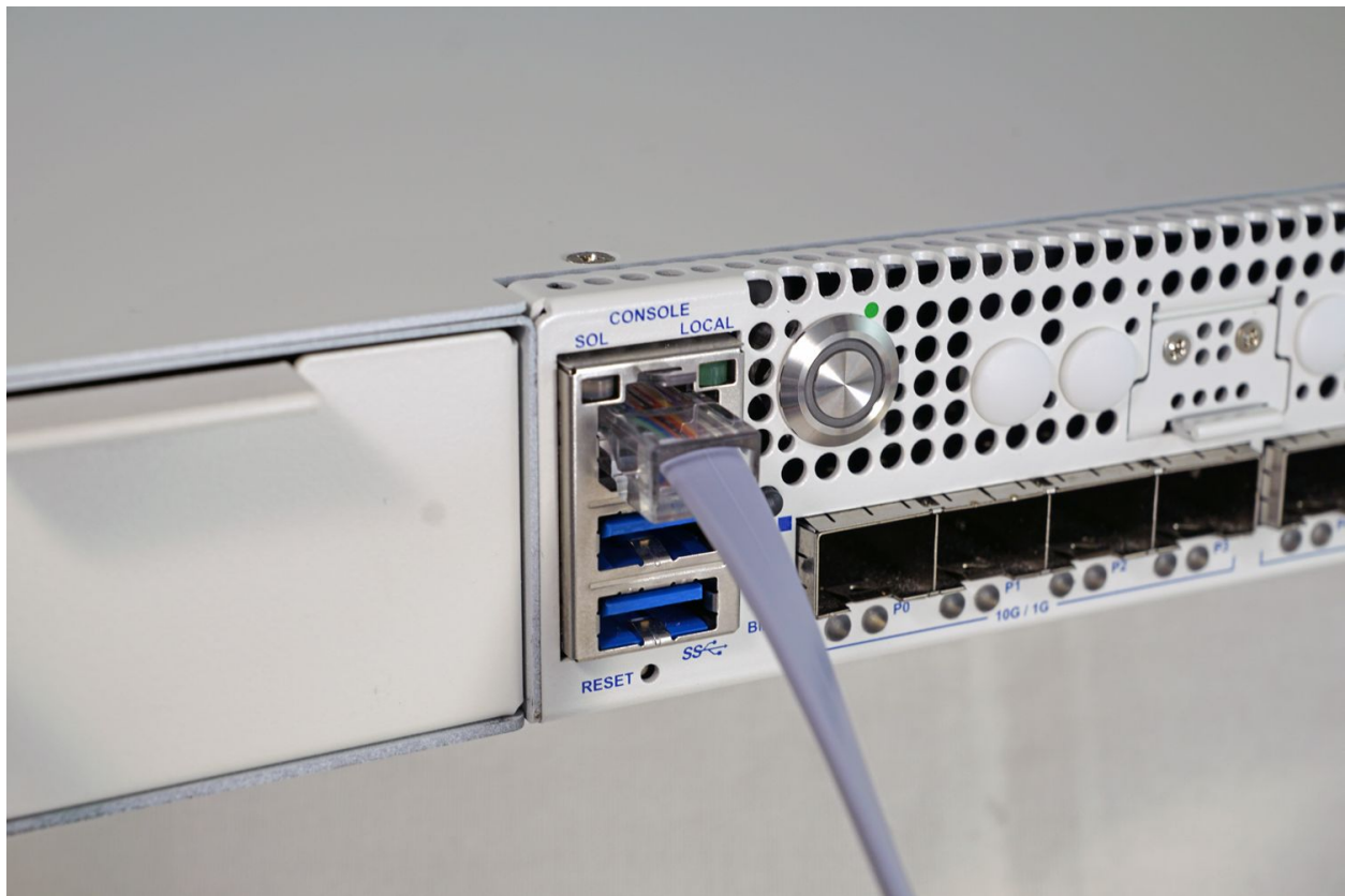
Fig. 1: Serial cable connected to RJ45 Console Port
