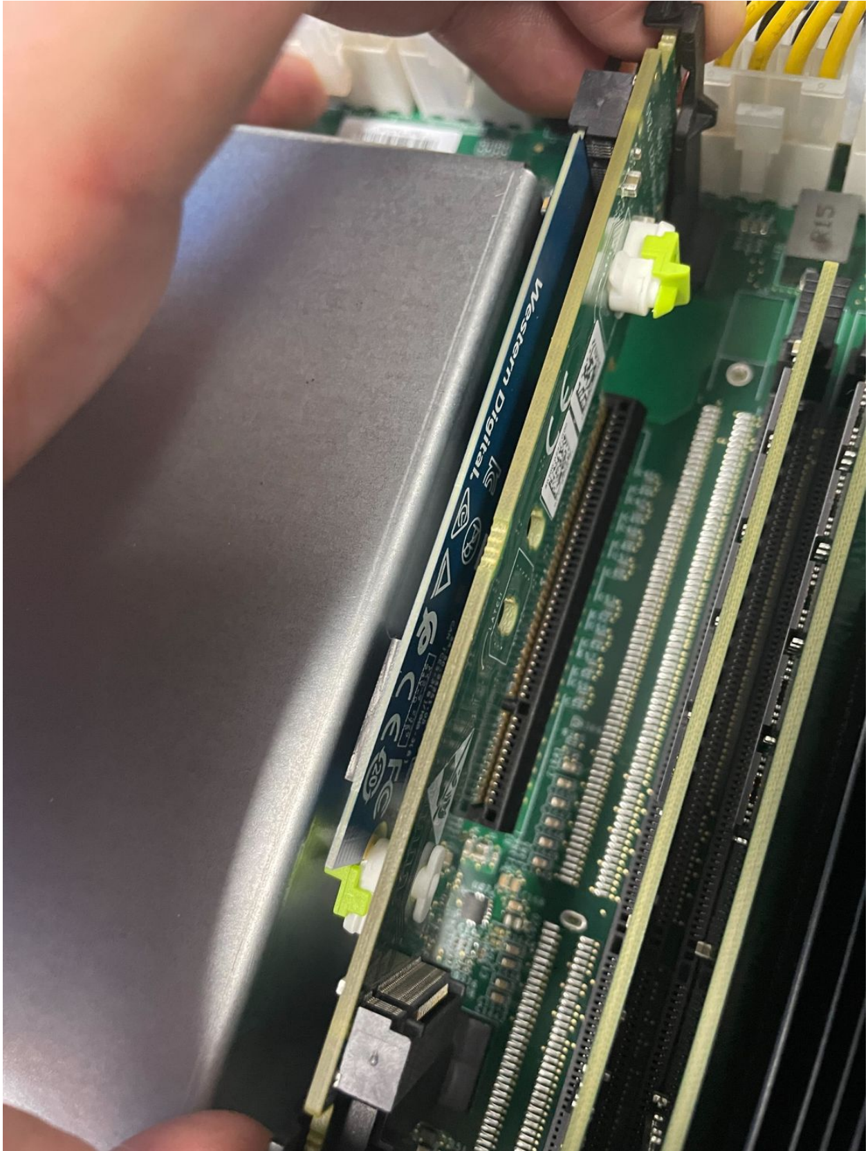
Fig. 16: Replacing the M.2 riser card
