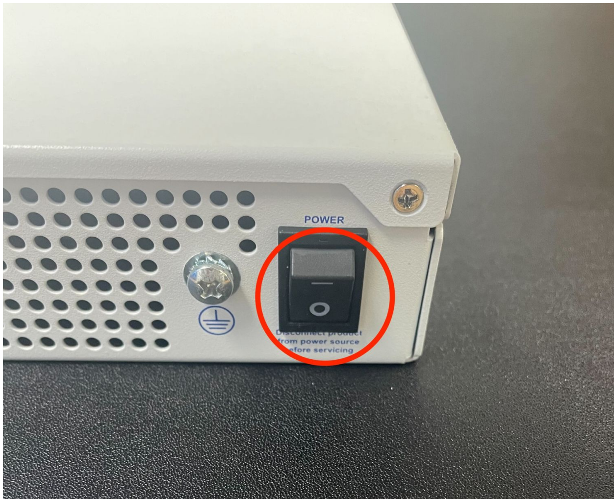
Fig. 1: Power switch (circled) in the off position
