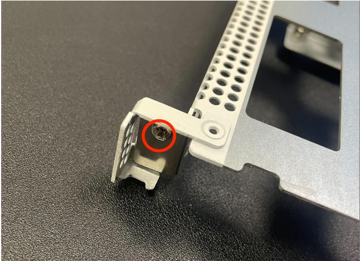
Fig. 14: Location of the full height add-on expansion card slot retaining screw indicated with a red circle
