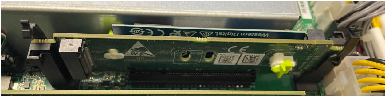
Fig. 11: M.2 NVMe riser card clips in the open position
