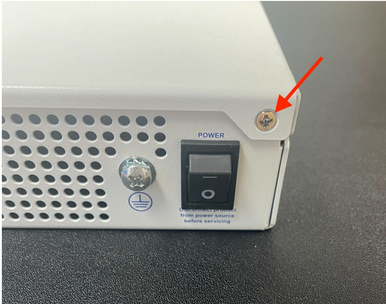
Fig. 28: Screw on the rear side of the unit at the right top corner, indicated with an arrow.
