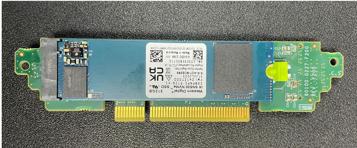
Fig. 14: M.2 NVMe riser card slot 2 with the add-on SSD installed
