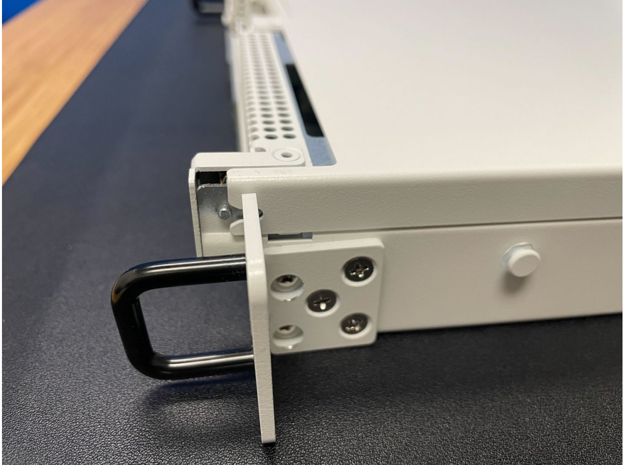
Fig. 19: Slide the top cover back toward the front panel
