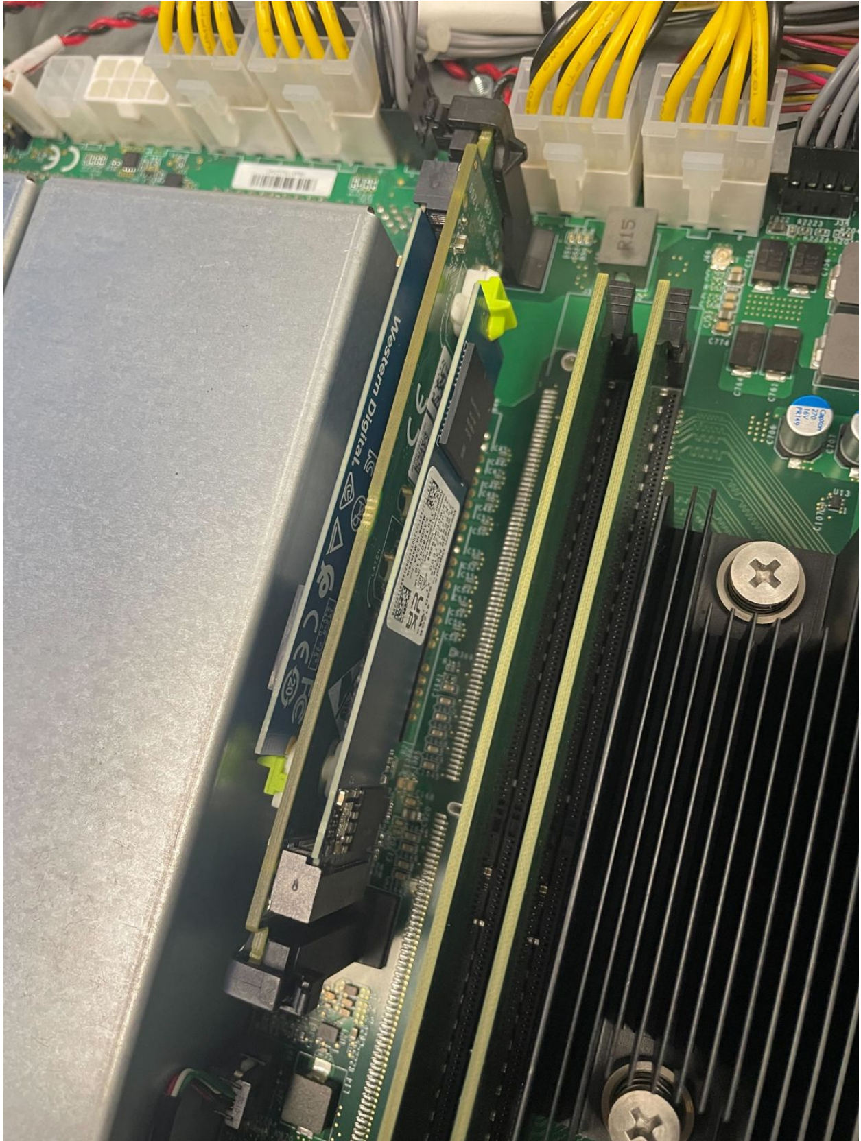
Fig. 17: M.2 riser card with two SSDs and riser clips in the closed position
