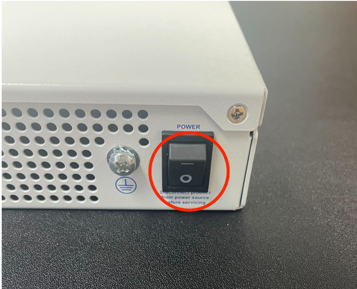
Fig. 1: Power switch (circled) in the off position
