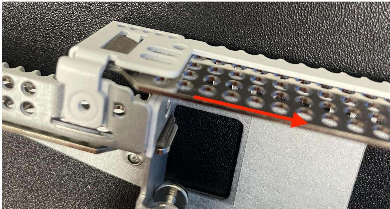
Fig. 15: Slide the expansion slot cover away from the center of the riser assembly
