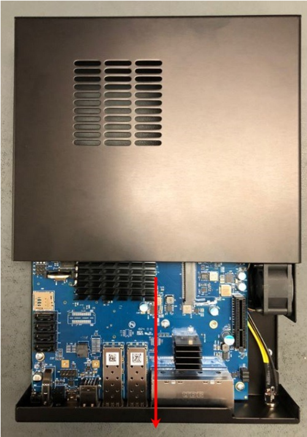
Fig. 11: Slide the Base of the System Away From the Lid
