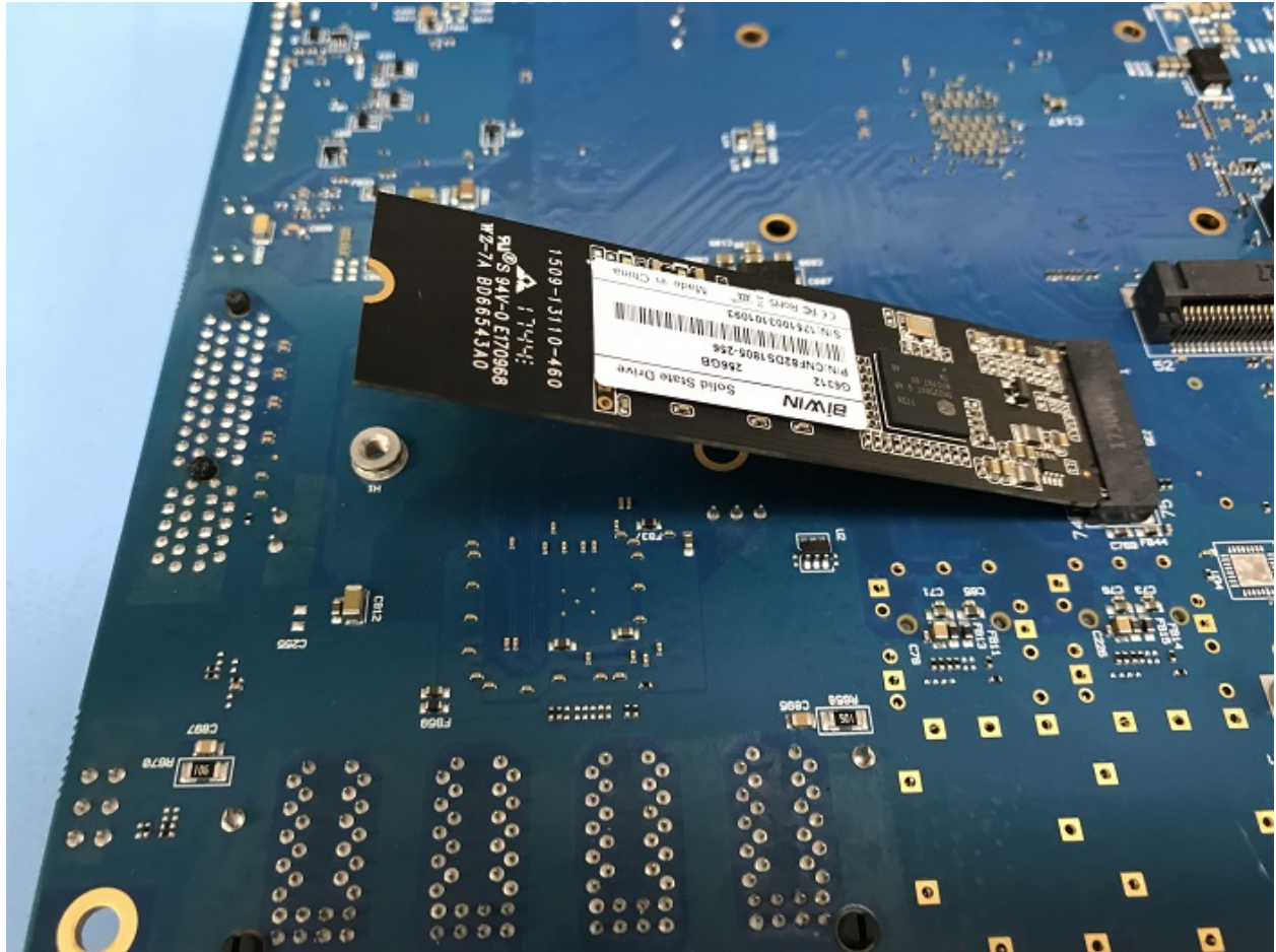
Fig. 15: M.2 SATA Drive Properly Inserted into the Slot
