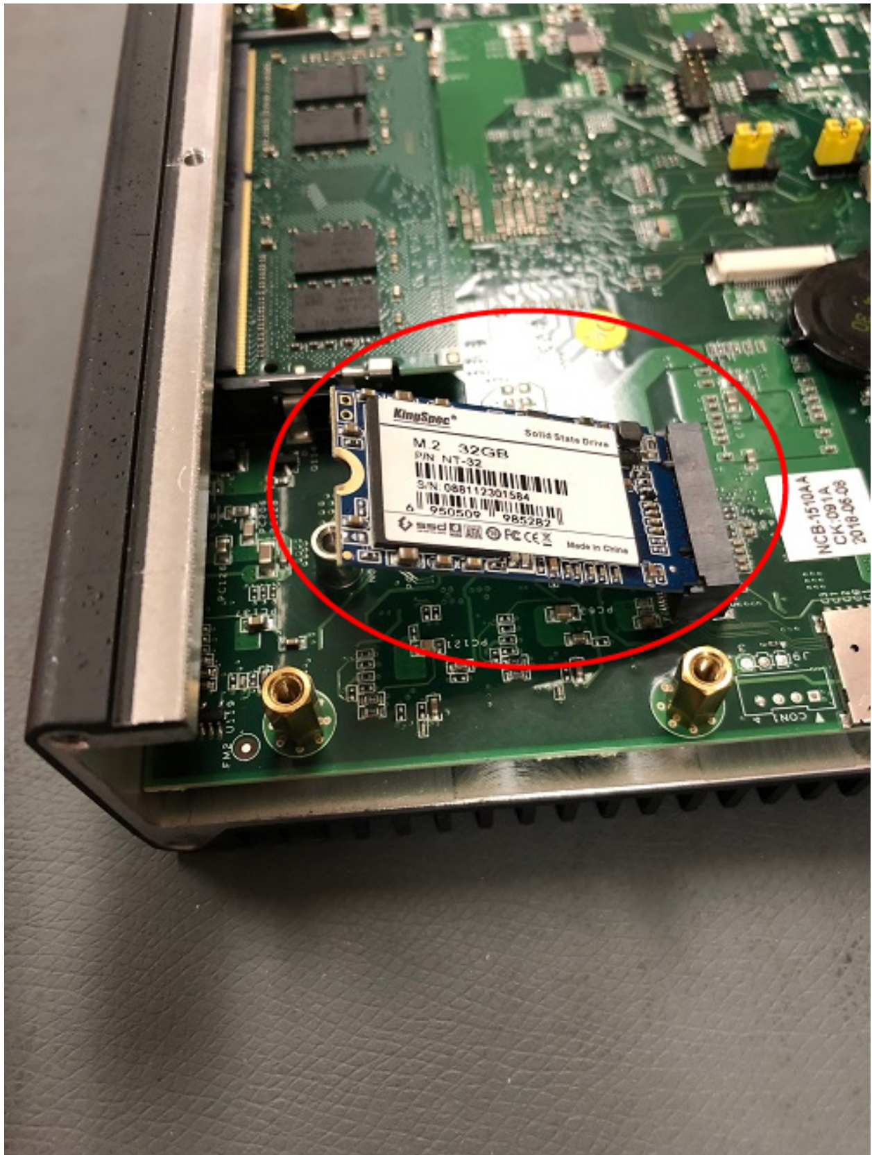
Fig. 9: Insert the M.2 SATA Drive at about a 30° Angle
