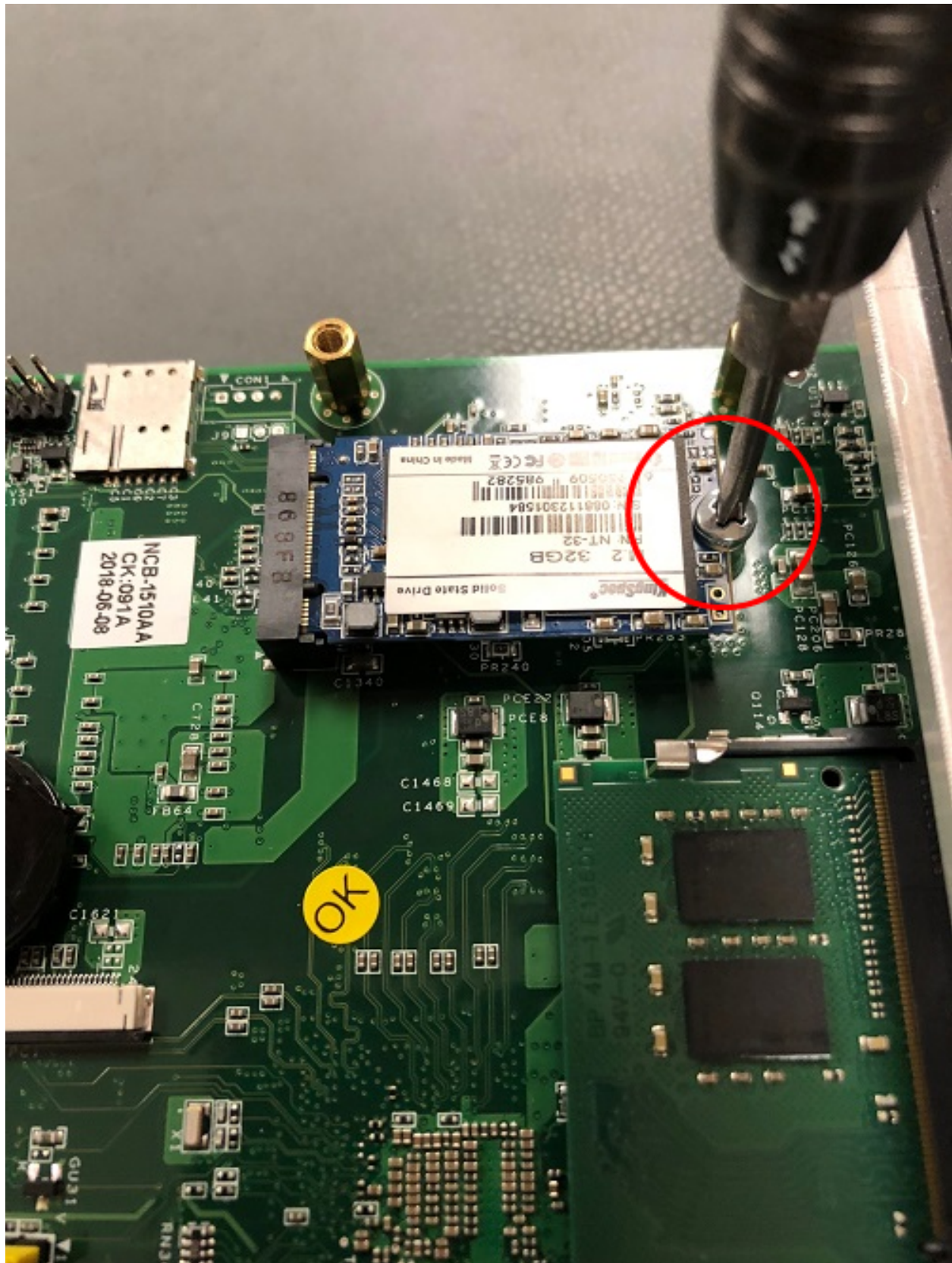
Fig. 10: Secure the M.2 SATA Drive
