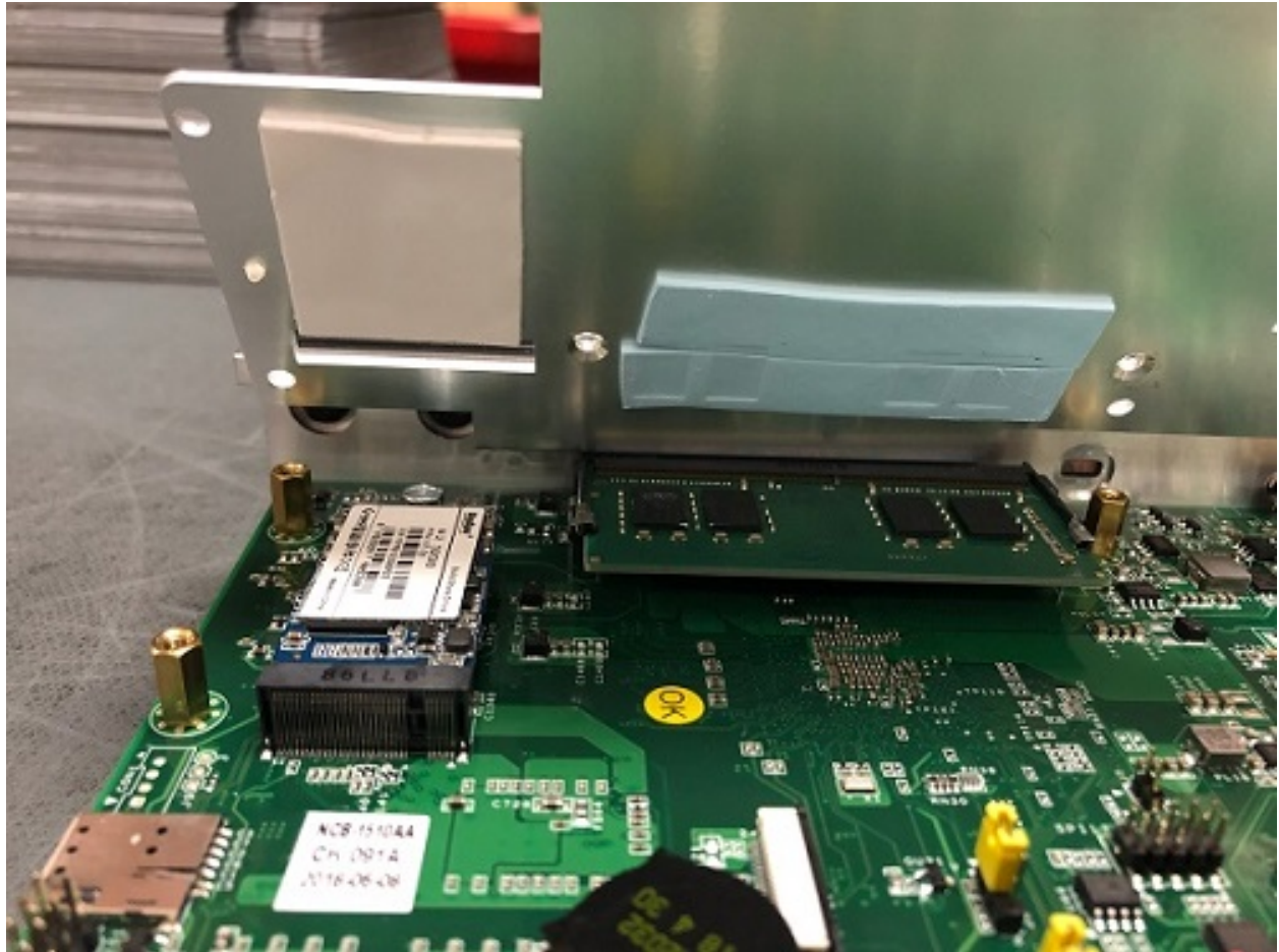
Fig. 16: Replace the heat sink
