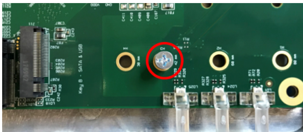
Fig. 6: M.2 SATA Location and Screw Close-up
