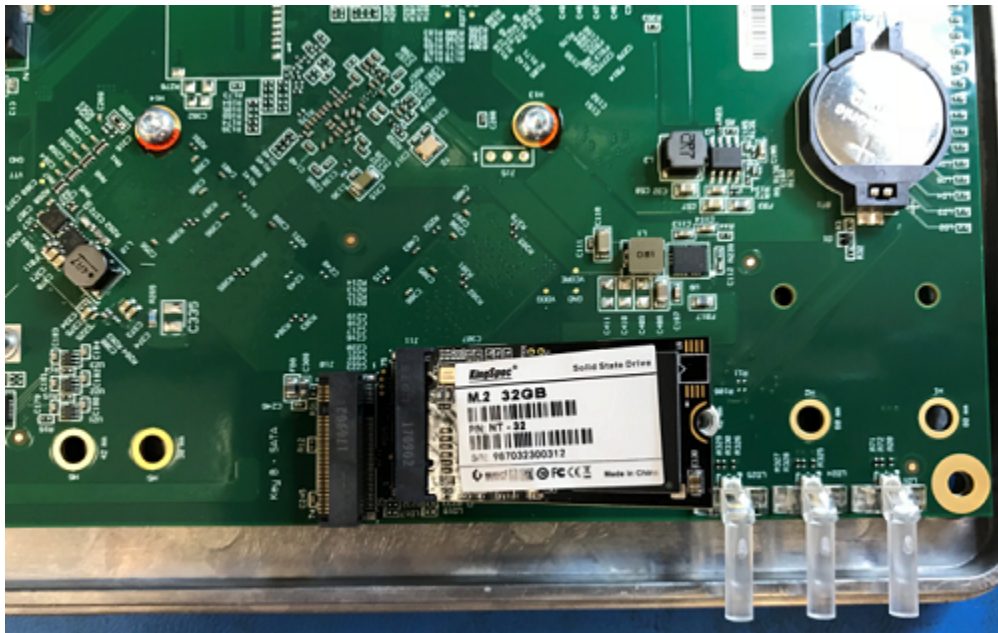
Fig. 7: Insert the M.2 SATA Drive at about a 30° Angle
