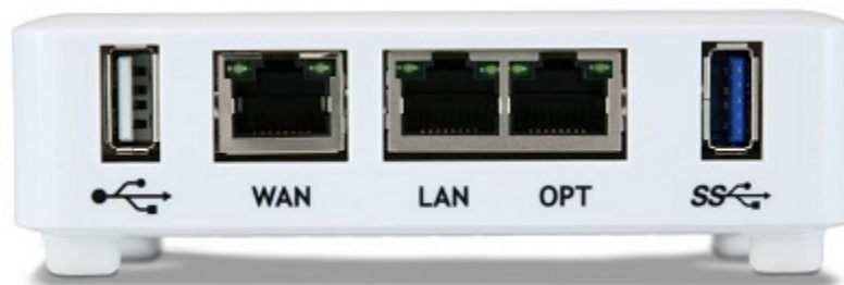
Fig. 12: Front view of the Netgate 1100 Firewall Appliance The items in this image are described by entries in Ethernet Ports and Other Front Ports .
