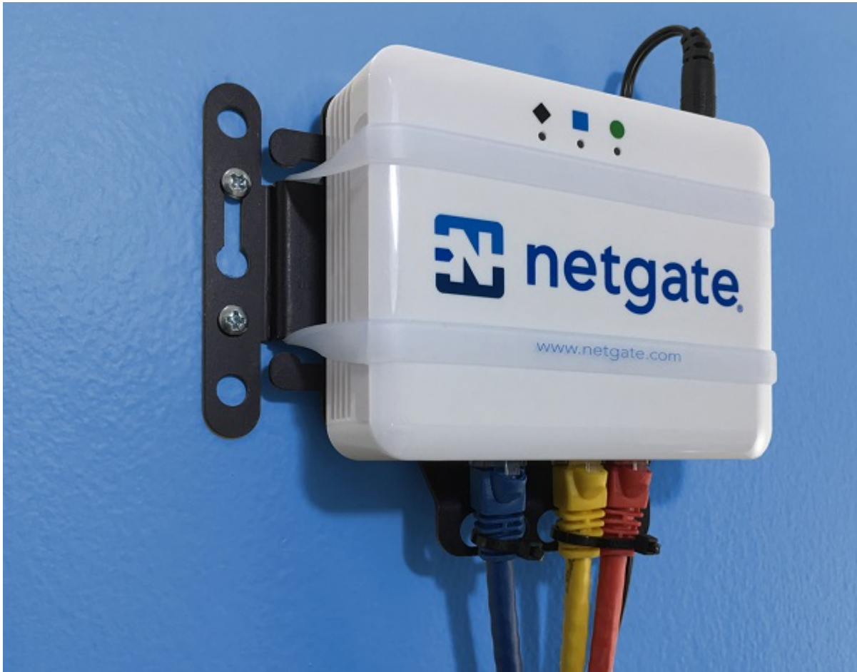
Fig. 9: An Netgate 1100 wall mount kit correctly installed
