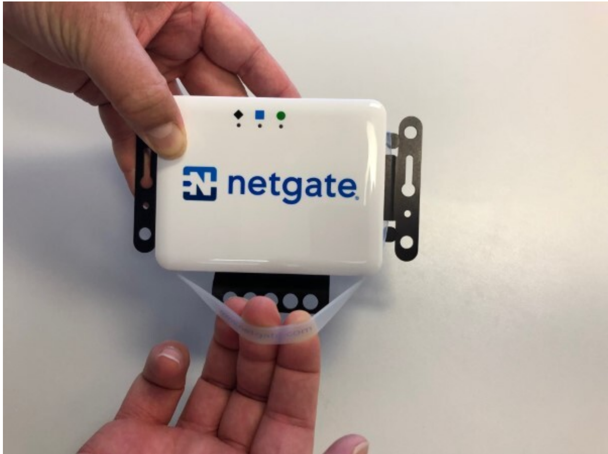
Fig. 6: Place the Netgate 1100 over the silver aluminum standoffs on the wall mount and pull one side of the silicone band over the Netgate 1100, then the other
