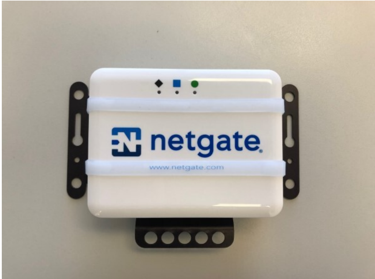
Fig. 7: When mounted properly, the Netgate 1100 should look like this
