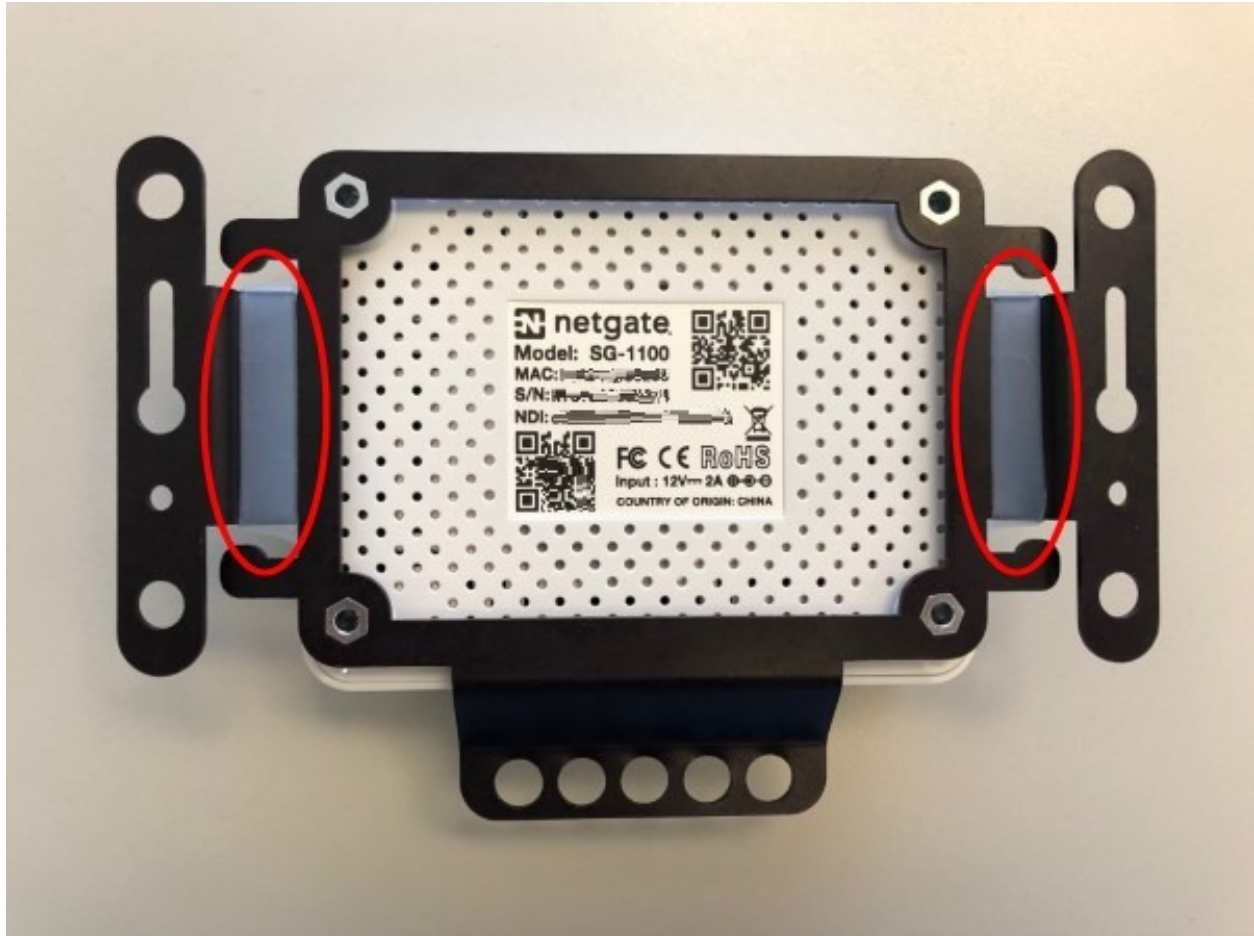
Fig. 8: Note the silicone band under the Netgate 1100 when installed correctly
