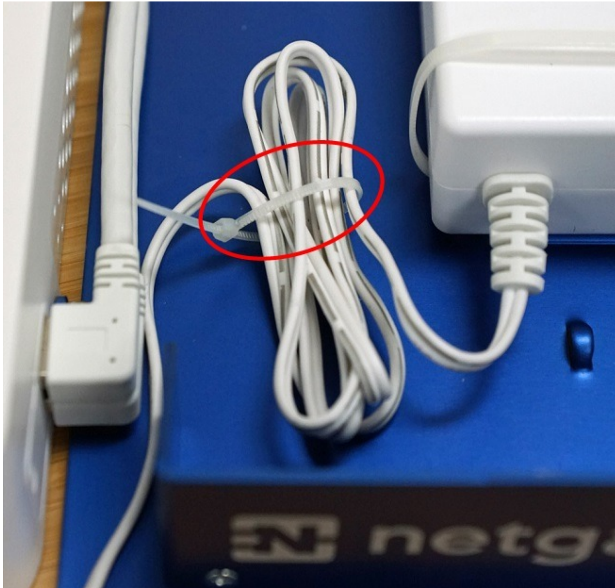
Fig. 12: Do not Cinch Down the Cable Tie Yet
