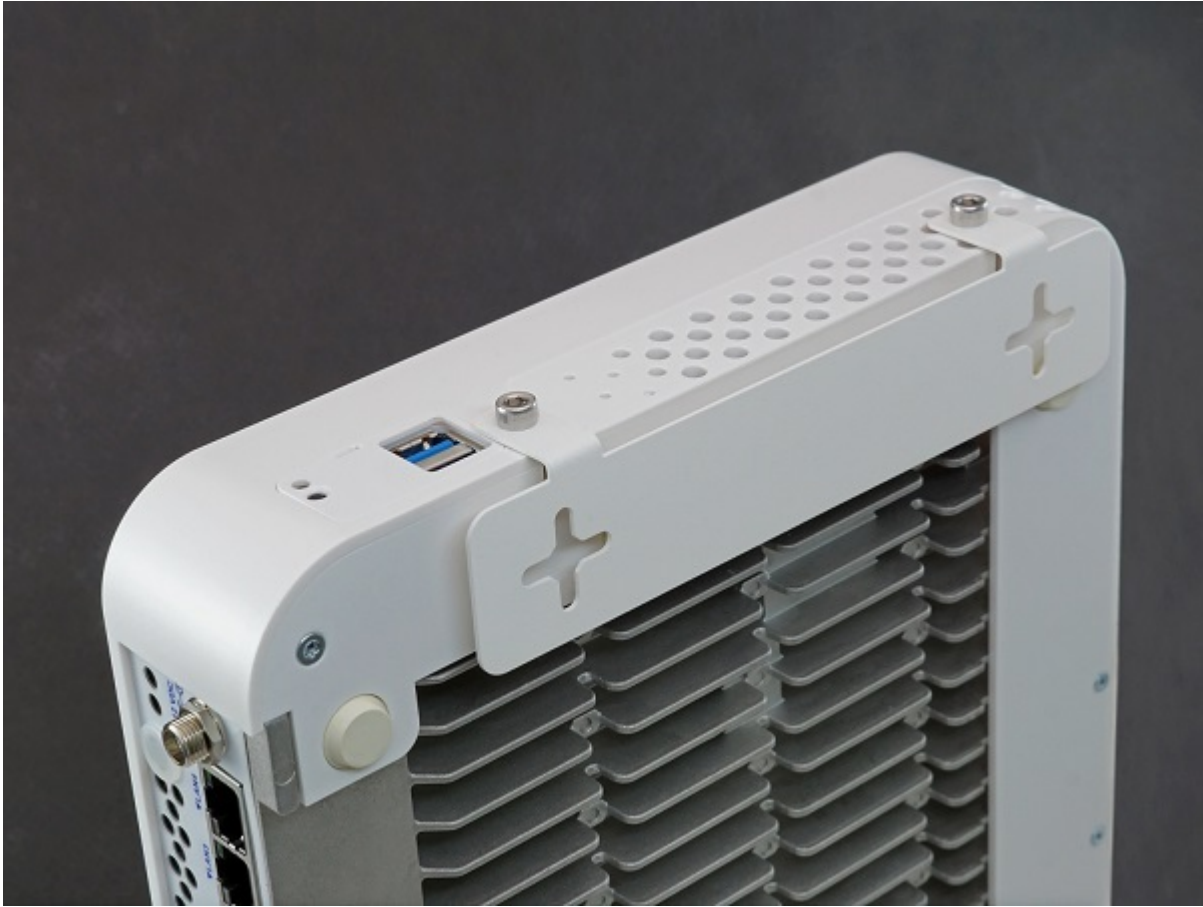
Fig. 18: The Netgate 6100 Inboard Wall Mount Orientation
