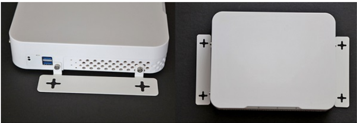
Fig. 19: The Netgate 6100 Outboard Wall Mount Orientation
