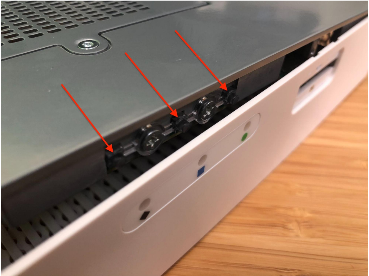
Fig. 46: Separating the lid from the LED guides
