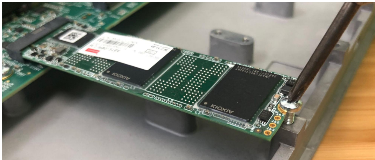
Fig. 49: Fastening the M.2 NVMe card retention screw
