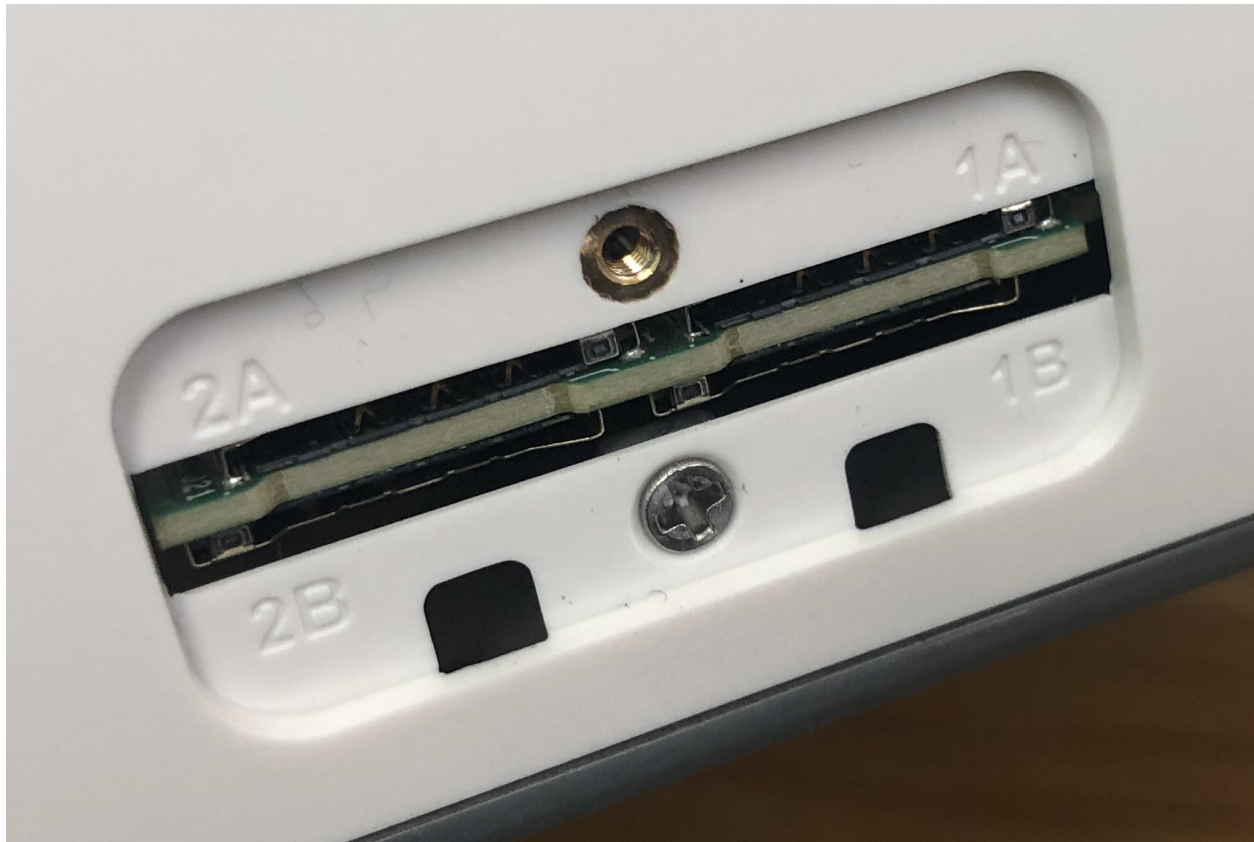
Fig. 4: Netgate 4200 SIM card slots and labels
