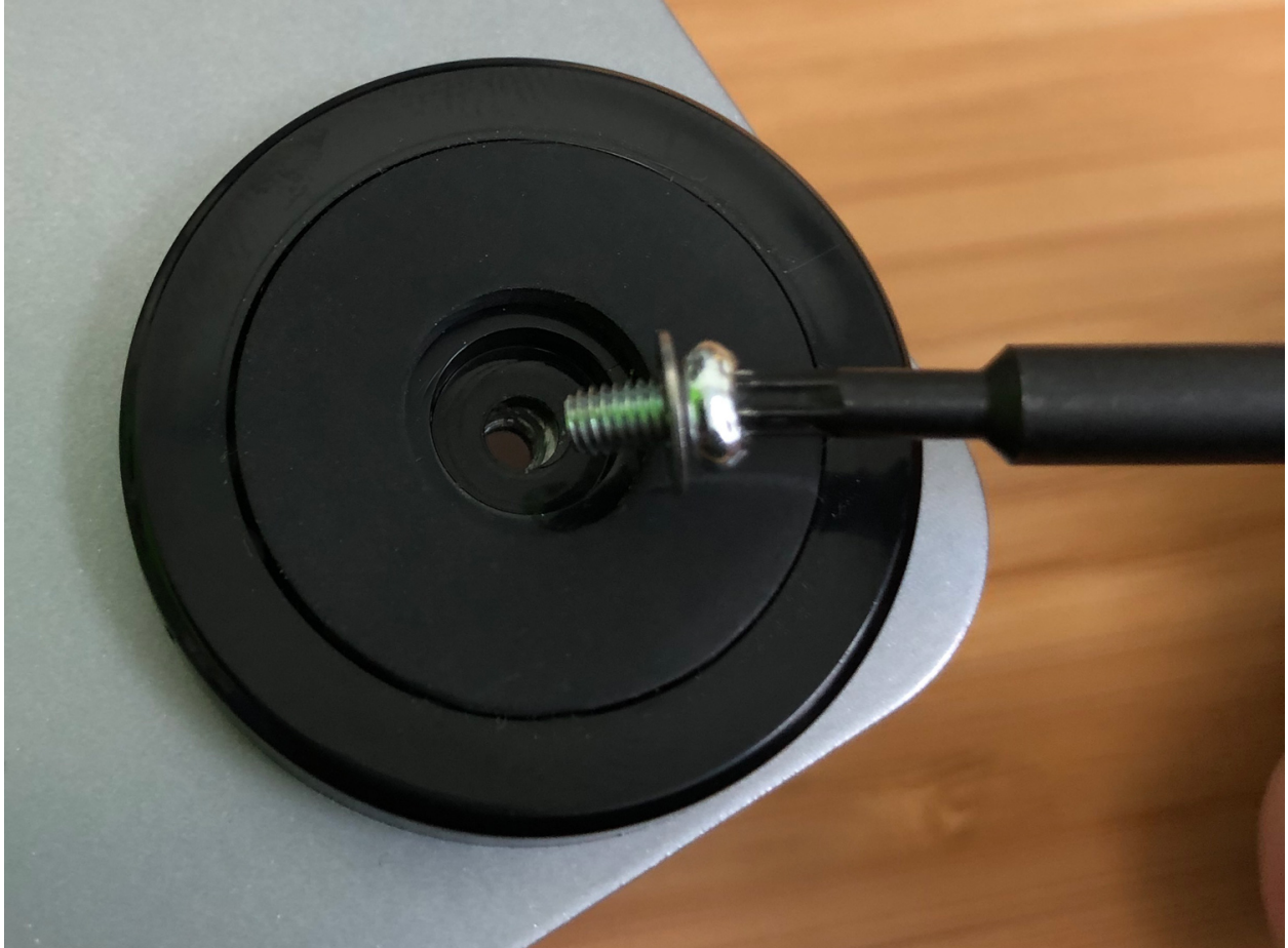
Fig. 42: Foot screw and washer removal
