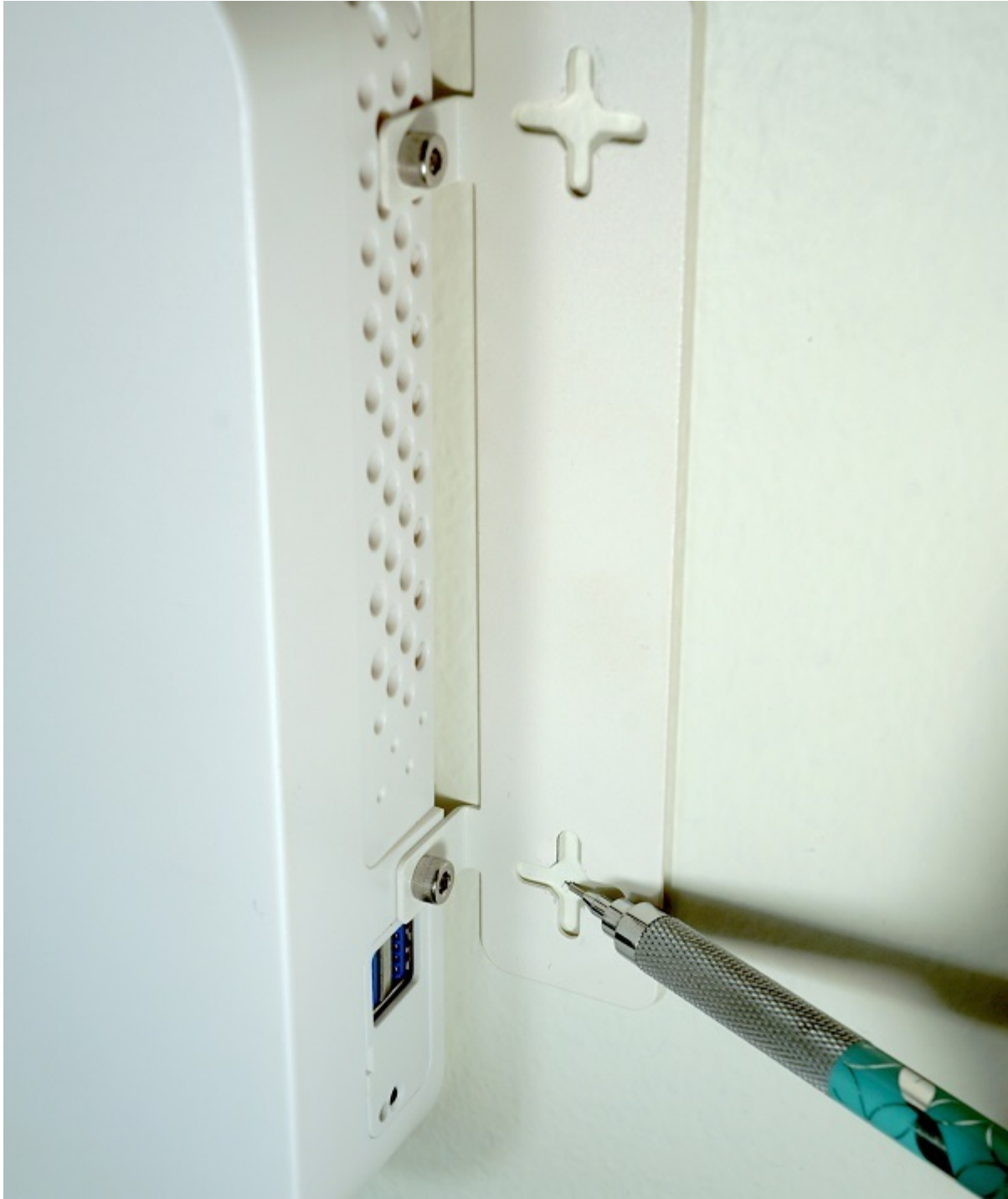
Fig. 8: Using the Wall Mount Bracket to Mark the Screw Locations
