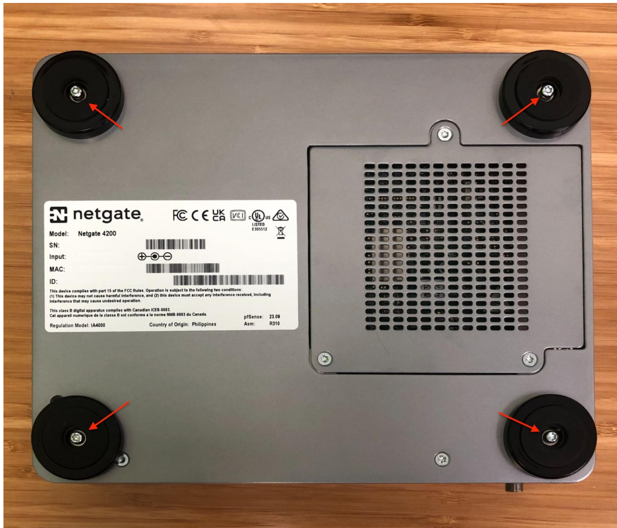
Fig. 41: Foot screw locations
