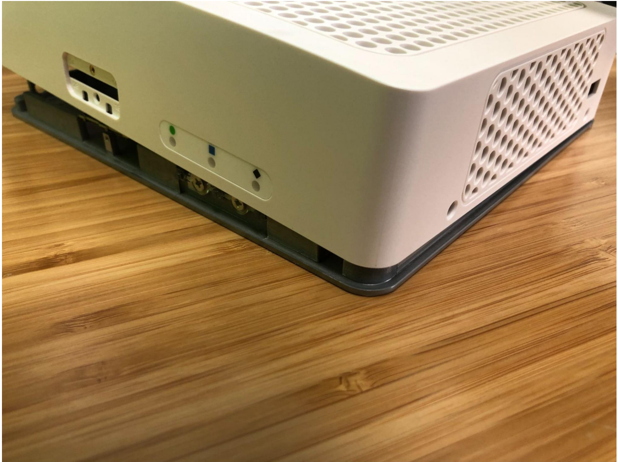
Fig. 51: Replacing the front part of the lid
