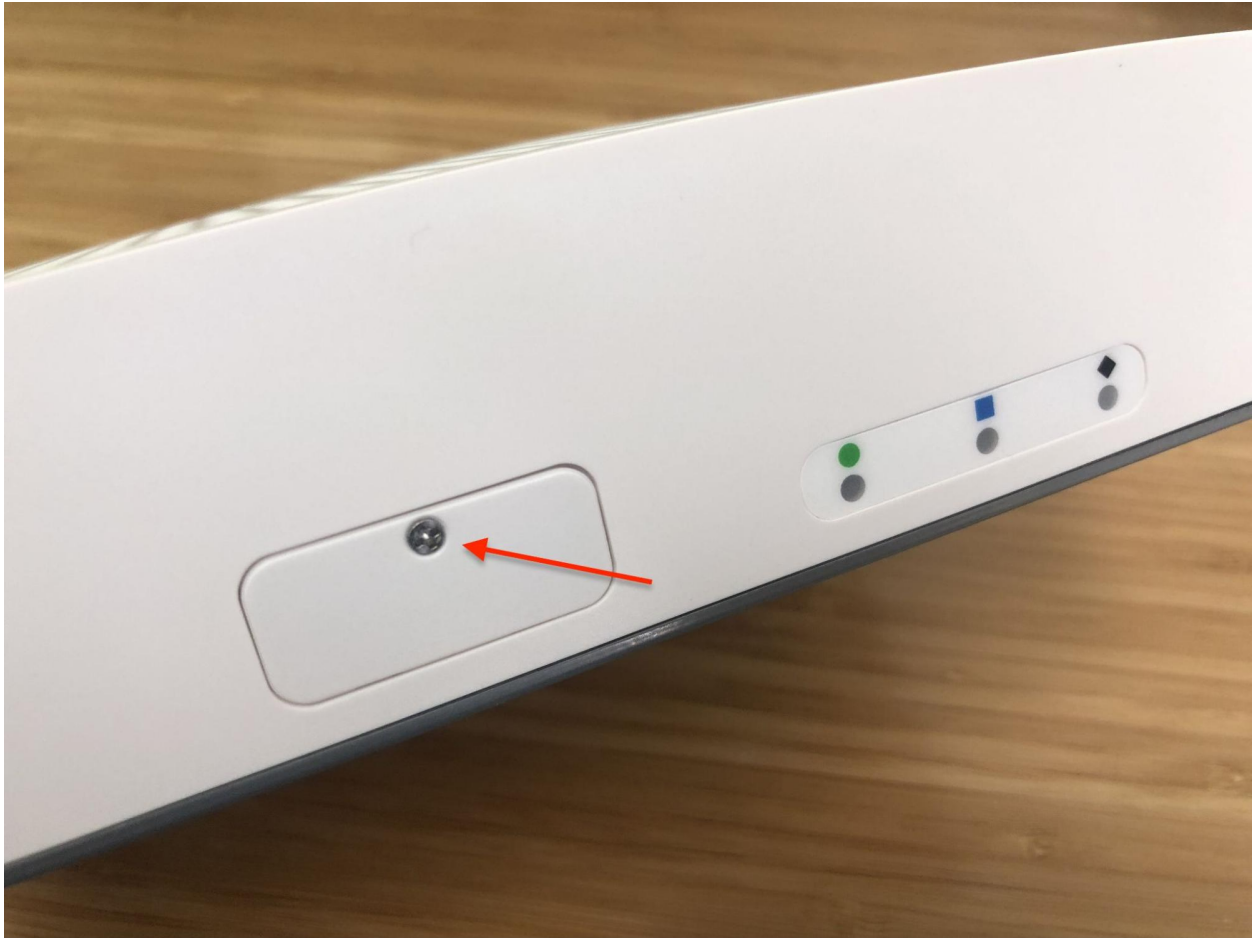
Fig. 39: SIM card slot cover screw location
