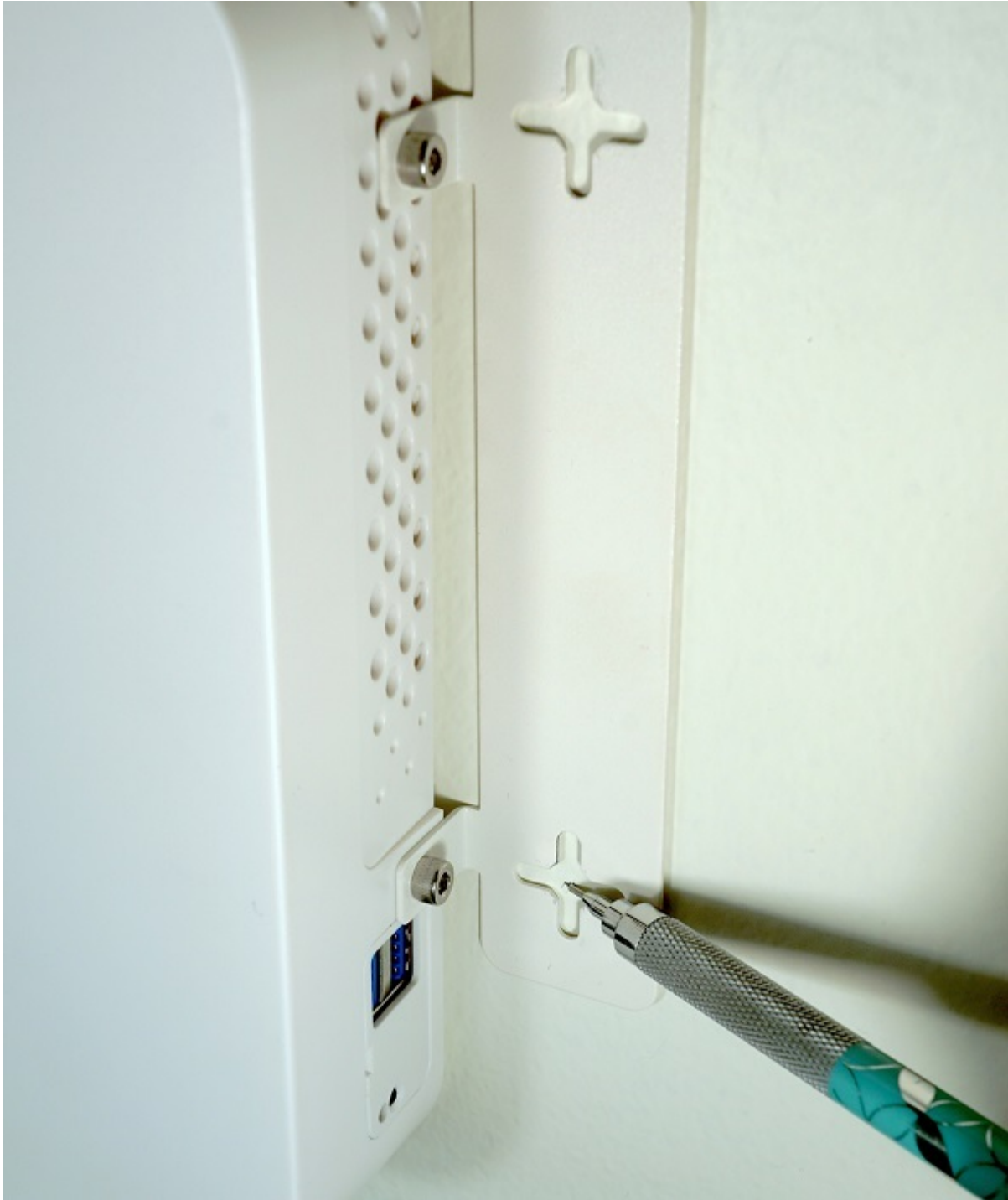
Fig. 20: Using the Netgate 6100 Wall Mount Bracket to Mark the Screw Locations
