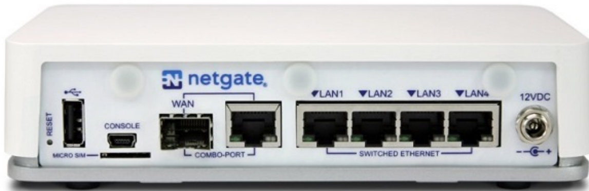
Fig. 1: Rear view of the Netgate 2100 Firewall Appliance The items in this image are described by entries in Routed Ethernet , Switched Ethernet , and Other Ports .
