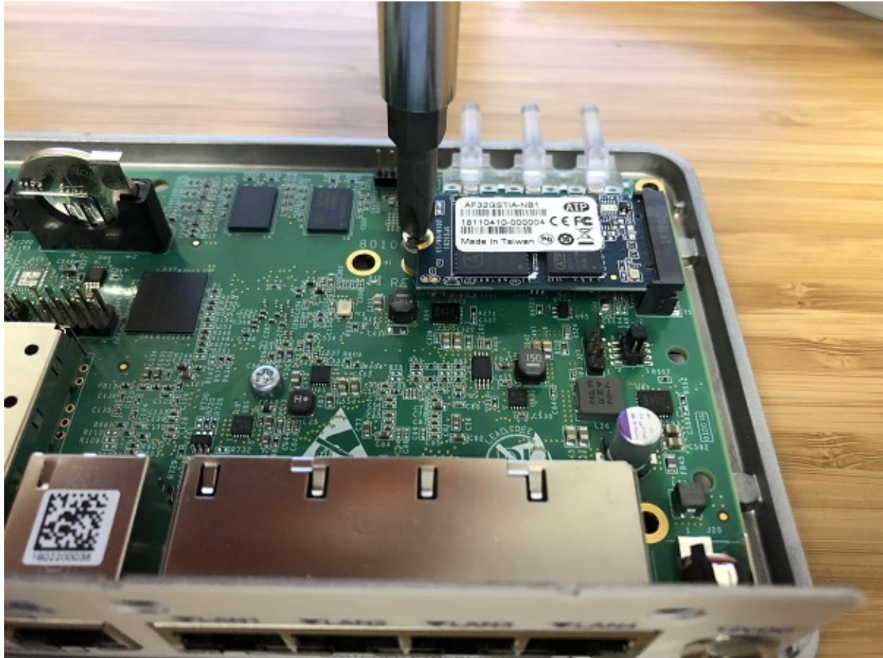
Fig. 4: The M.2 SATA Drive Installed
