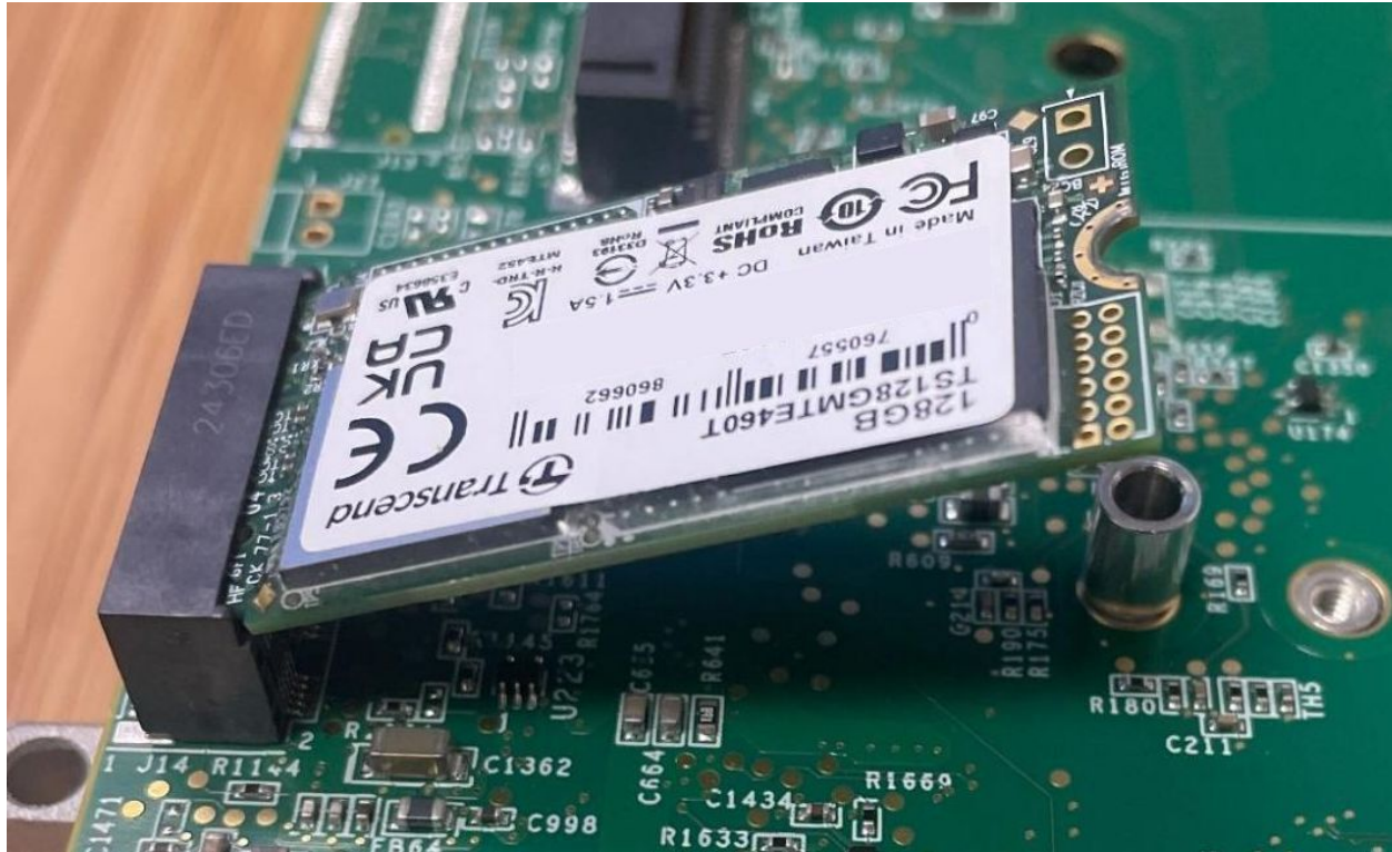
Fig. 31: Inserting the SSD into the M.2 socket at an angle
