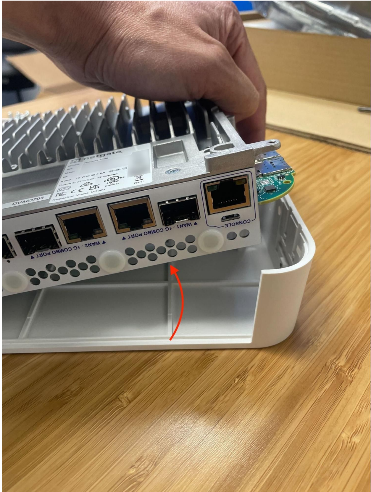
Fig. 29: Removing the Netgate 6100 chassis from the lid
