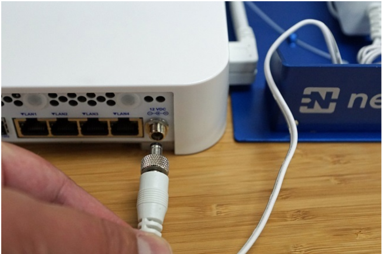
Fig. 13: Do Not Put Tension On The Cable. The Cable Should Have Enough Length to be Removed Without Excessive Tension.
