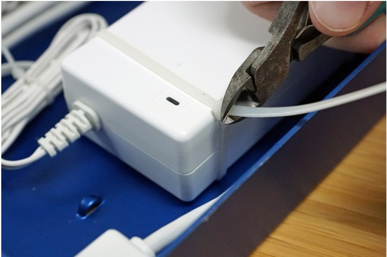
Fig. 14: Cut the Excess Cable Ties
