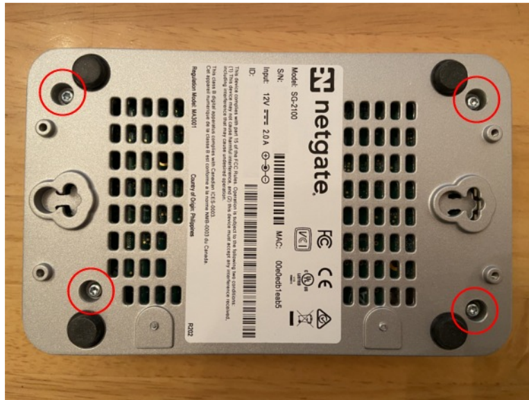
Fig. 1: Removing the Netgate 2100 Case Screws
